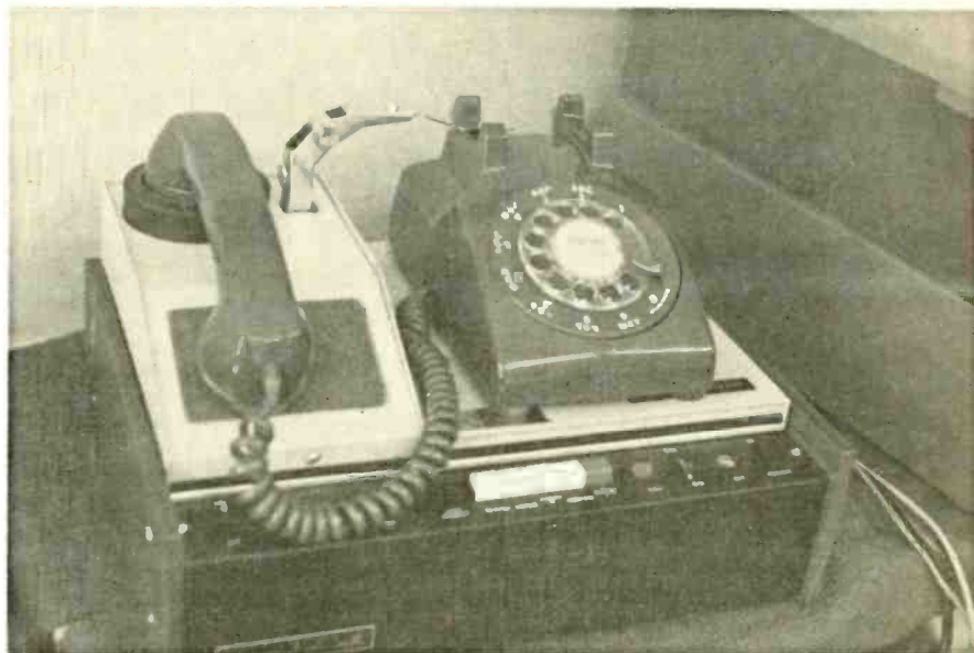
THE GEMINI , by Record-A-Call uses physical lift unit and offers a choice of acoustic or inductive coupling so there is no need for direct electrical tie to phone line.
