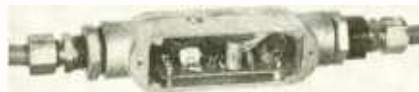
WWVB PREAMP is in the loop antenna. It should be completely shielded.
