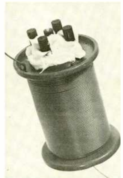
EXPERIMENTAL SUPER-LOOPSTICK is shown less shield. Rods are 5/16-inch long. Figure of merit is around 2. Resonating capacitor is around 235 pF.
